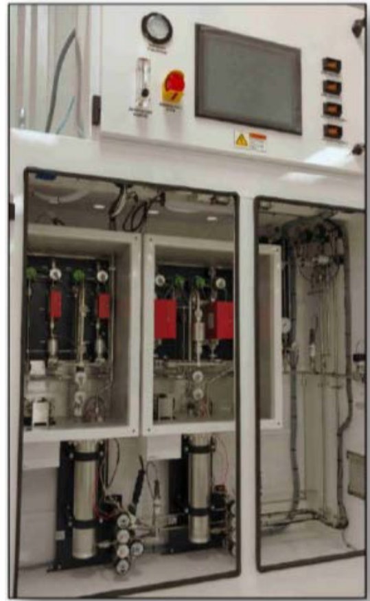
The VaporGen™ i2000 with 2 SMRs and 4 Vapor MFCs
